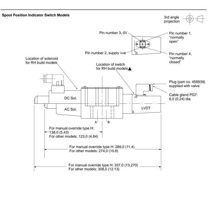
▲ For LH models ("L" in model code location ③) solenoid and switch locations are reversed
